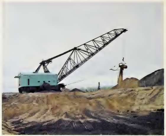
This giant walking dragline at Wabamun strip mines coal for use as fuel in the Calgary Power generating plant. It is capable of taking 35-cubic-yard "bites" from the open pit mines.
